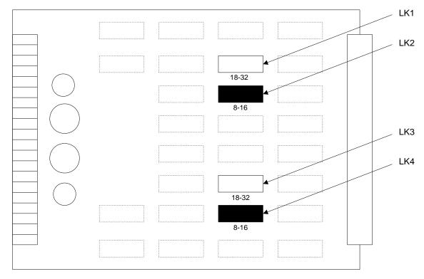
Figure 4.1 - Location of link headers for selecting the display mode
